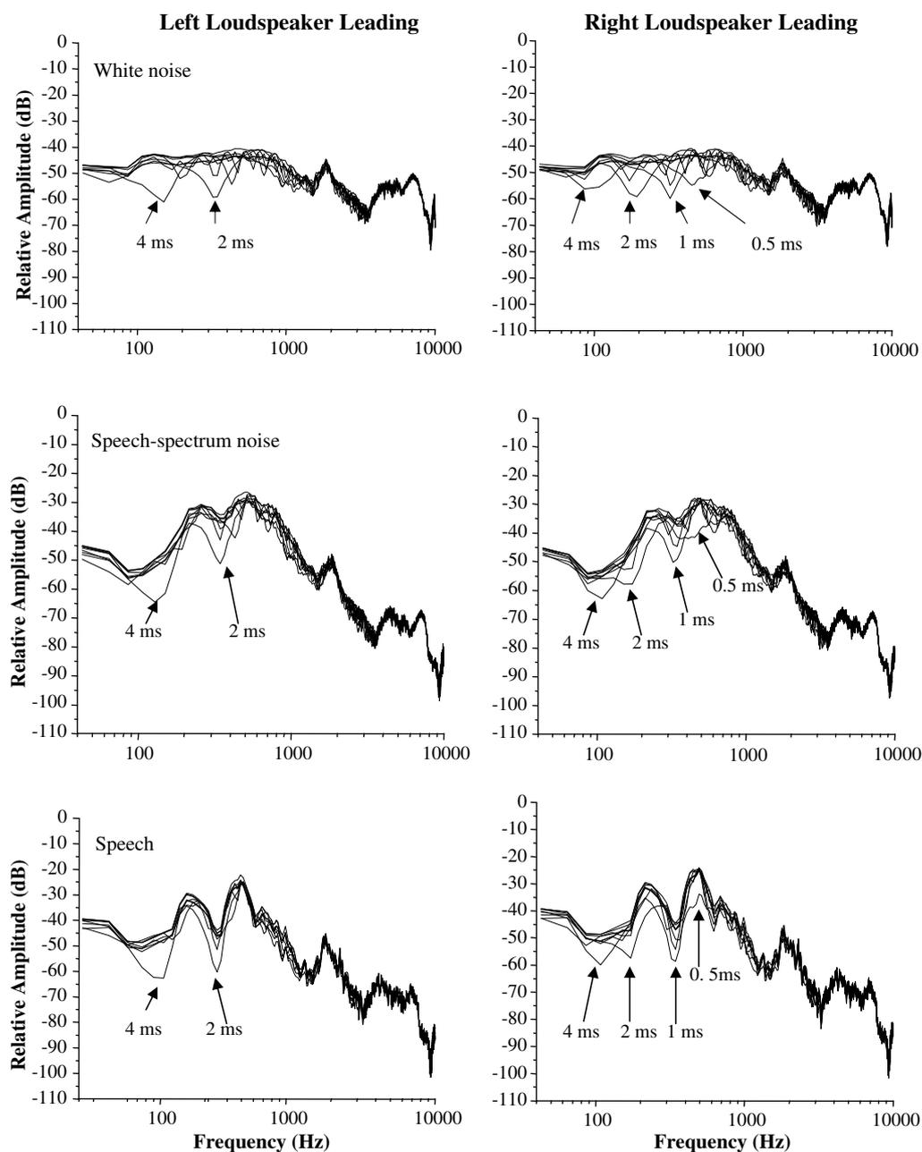
**Fig. 10.** The spectra of white noise (top panels), speech-spectrum noise (middle panels), and target speech (bottom panels), which were recorded at the right ear of the Knowles Electronic Manikin for Acoustic Research (KEMAR) placed at the participant's position in an anechoic chamber. Each curve in each panel represents the spectrum of one of the 3 types of sounds (white noise, speech-spectrum noise, speech) at a particular inter-loudspeaker delay between two identical stimuli.
