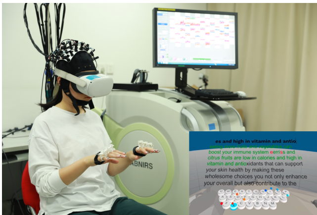
Figure 8: Settings of the study 2. The participant is engaged in air typing while wearing functional near-infrared spectroscopy (fNIRS) devices.
